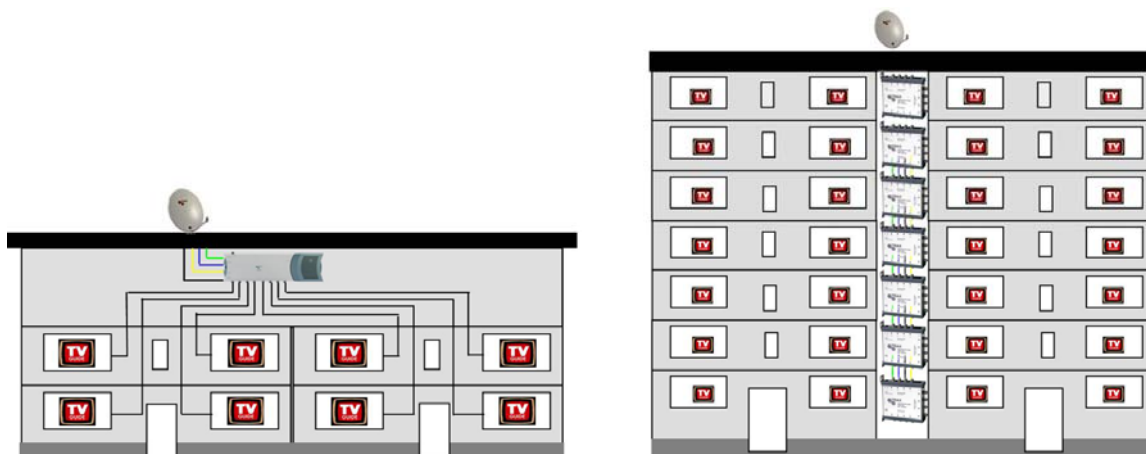
Fig. 2: Star-topology versus trunk-topology
